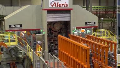
Aluminium strip produced with the innovative Alcoa Danieli Micromill process which offers improved mechanical characteristics: see possible production of 7xxx alloys to compete with steel.
