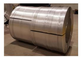
Endless aluminium and copper hard-alloy rod production; less than 3 hours from ingot to finished coil with 3 operators
